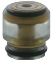
CAUTION Nearly empty cartridge seal - this seal should have been replaced when the oil level reached 1/2 of the original volume.
