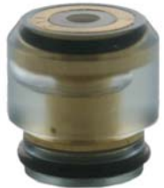
Cartridge seal with an acceptable bubble - this seal is okay to use.
