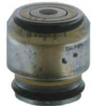
CAUTION Cartridge seal with contamination - this seal should be replaced.
