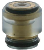
Cartridge seal with an acceptable bubble - this seal is okay to use.
