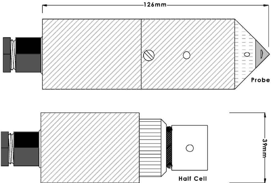
Fig.1 - UCP 1A Contact Probe
