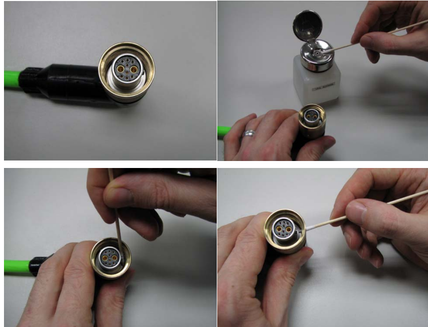
Figure 14. Cleaning the o-ring surface with IPA
