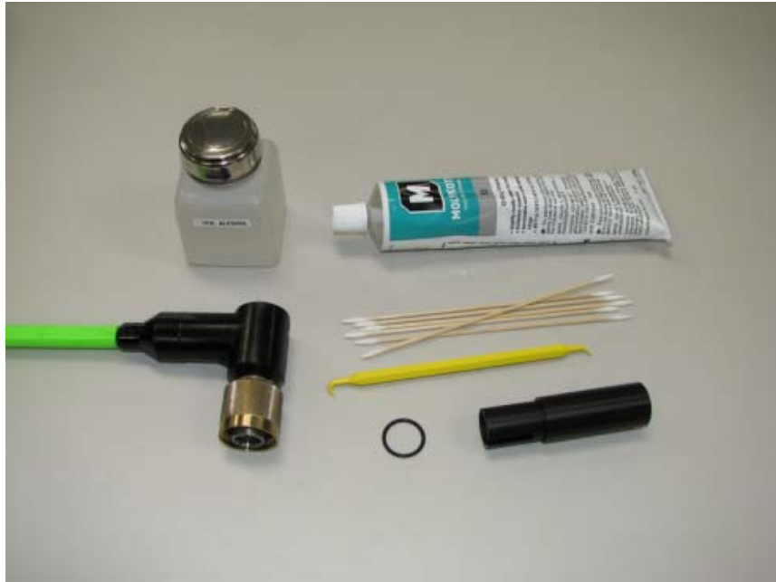
Figure 12. Items required for SEA CON CCP o-ring replacement
