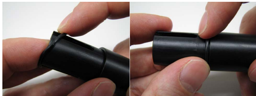
Figure 16. Fit the o-ring onto the DOIT and slide it to the end
