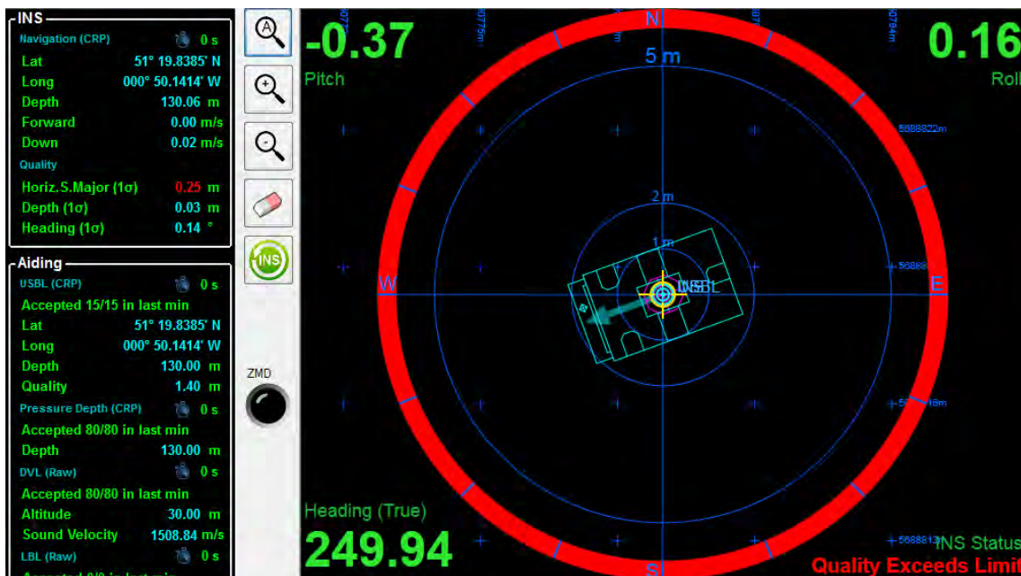
Figure 9-13 Navigation Quality Limits Exceeded
