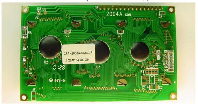
Seetron supplies a 14x1 "Berg strip" for displays that use a single row, and a 2x7 "Berg strip" for displays that use double-row connection. We will use the 1x14:
