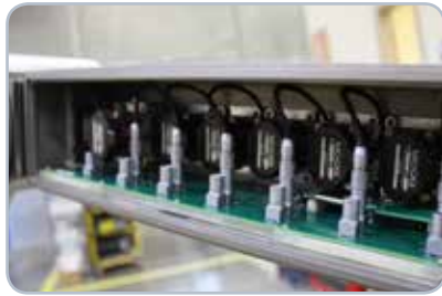
In-arm electronics are located in the forearm, increasing system reliability and minimizing electrical connections.
