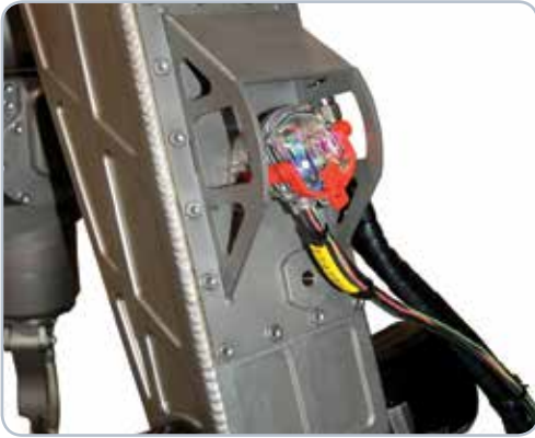
Colored diagnostic lights in the connector head indicate the status of electrical power delivery to the arm, master controller transmission to the arm, and arm responsiveness.
