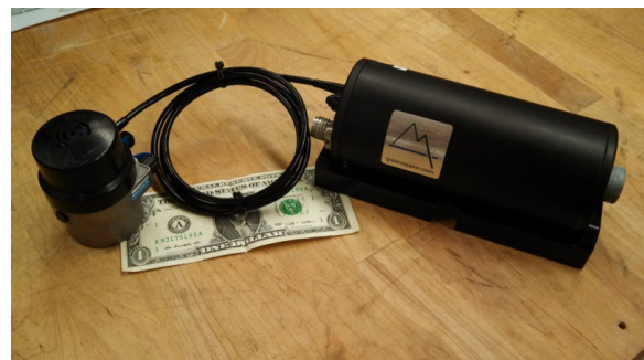
Illustration 4: Trittech Micron mechanically scanned imaging sonar with Greensea embedded feature-based navigation system and MEMS-based INS.
