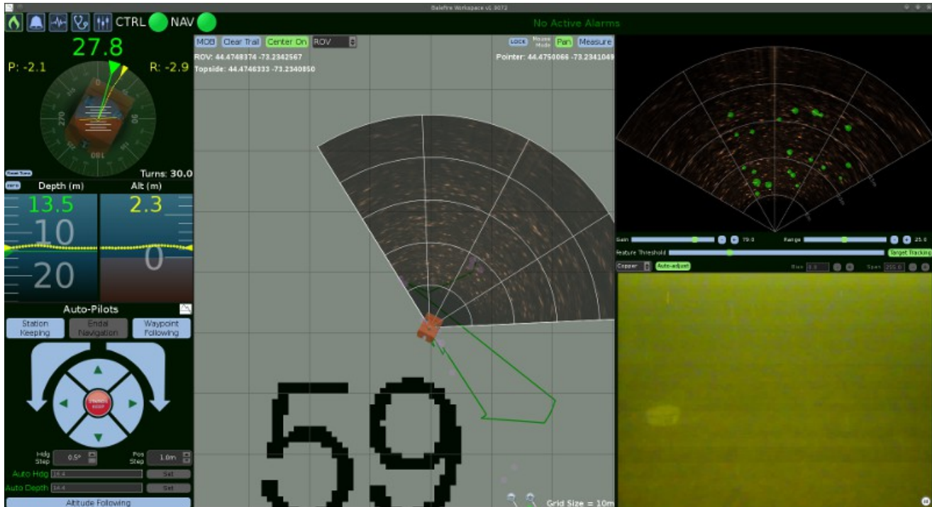
Illustration 12: Greensea's Balefire ROV control system interface with feature navigation active utilizing a Tritech Gemini multibeam imaging sonar.
