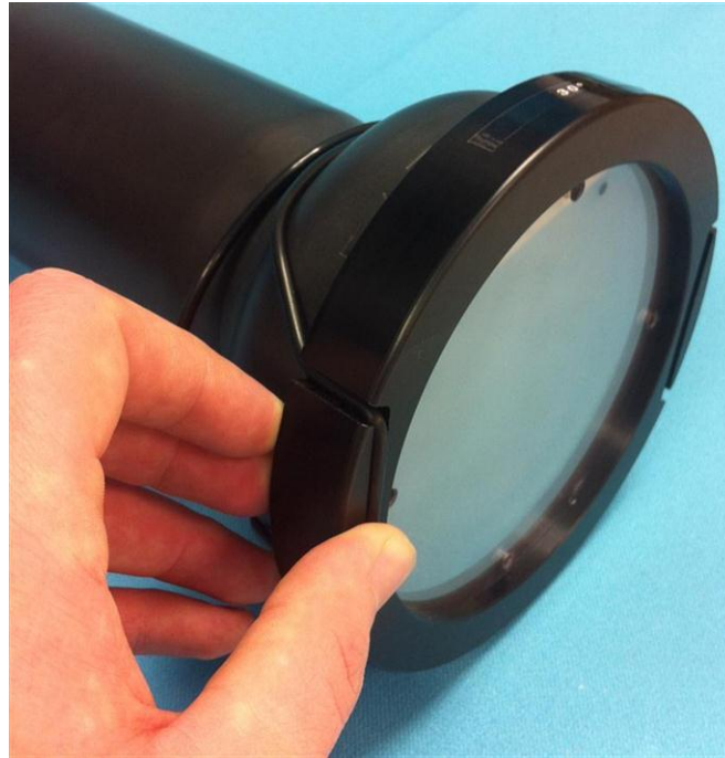
Figure 32. First O Ring fitted to Diffuser Face
