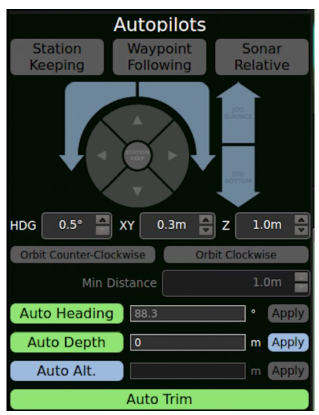
The autopilot functions are located directly beneath the vertical velocity gauge.
