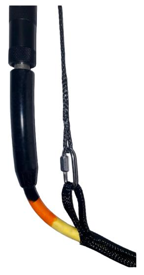
6. Make sure the strain relief cable connections are secure so that all of the load is carried by the strain relief and there is no load on the tether connection.
