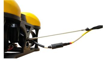
When working in an area where there is a chance the tether can become snagged on a protruding object, the connection can be wrapped with tape to prevent a protruding object from passing through the space between the tether and the strain relief cable.
