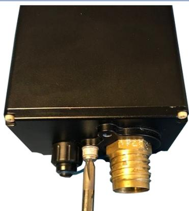
**Step 1:** Remove the spent or damaged sacrificial anode from your sonar with a cross head screwdriver.
