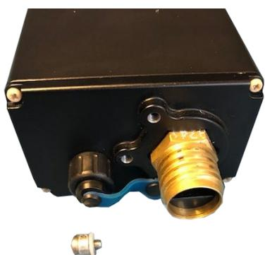
**Step 3:** Fit to the sonar and tighten up the screw.
