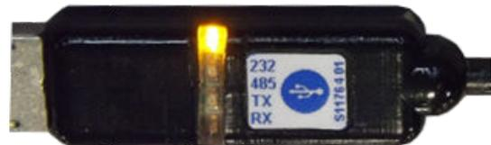
*A USB to serial Converter indicating that has established communications*
