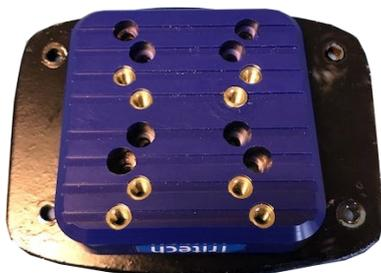
**Step 1:** Place the adapter onto the vehicle or mounting plate and place 4 of M4 x 10 screws into the required mounting holes.
