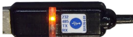
*A USB to serial Converter indicating that it is establishing communications*
