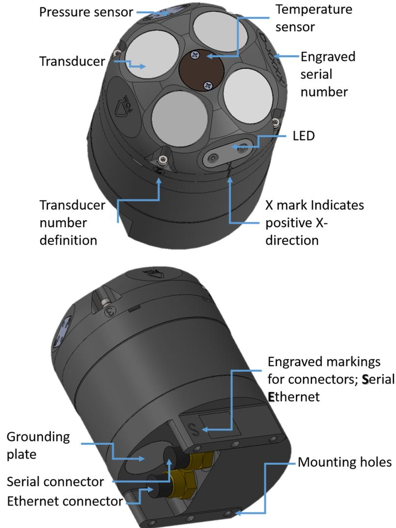
**Displayed is a Shallow Water 1 MHz DVL (DVL1000-300m) and differs from the deep water variants by having the Grounding Plate**
